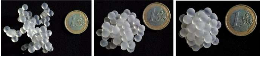
Fig. 27 3D-printed aggregates with N = 74 monomers, each with radius r = 2.5 mm. Fractal dimension values equal to 2, 2.5, and 2.8 in the left, centre, and right panels, respectively
